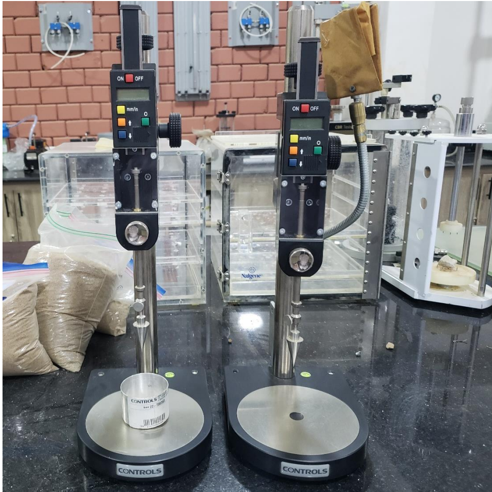
Plate 4: Digital cone penetrometer for Liquid Limit determination
