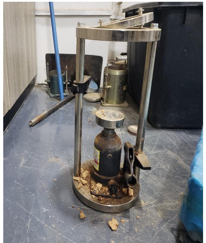
Plate 5: Typical apparatus set for Proctor compaction test
