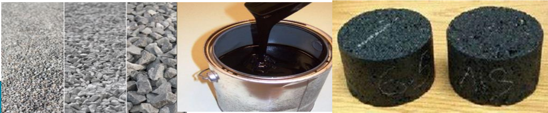
Plate 7: Aggregates, bitumen and test samples
