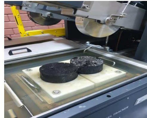
Placing of resized sample in testing mould
