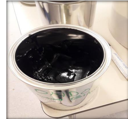
Extracted bitumen samples
