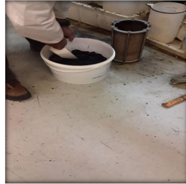
Mixing the Bituminous sand with Di-chloroethane
