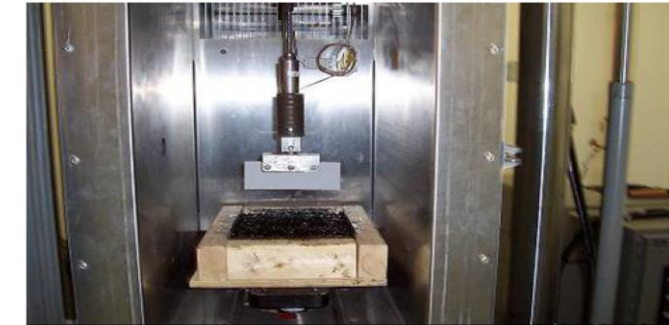
Fig 3. Blade resistance workability test apparatus [9]
