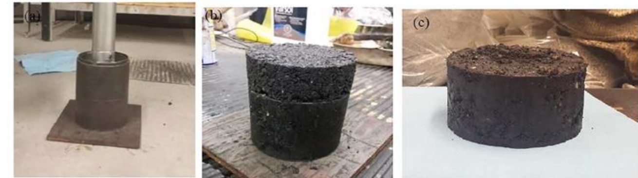
Fig 4. Procedure of the adhesiveness test: (a) CMA compaction on top of HMA, (b) sample extrusion, (c) weighing the remnants after inverting the sample and measuring the separation time
