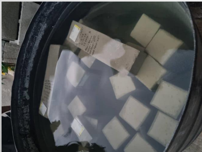
Curing of Concrete Beams
