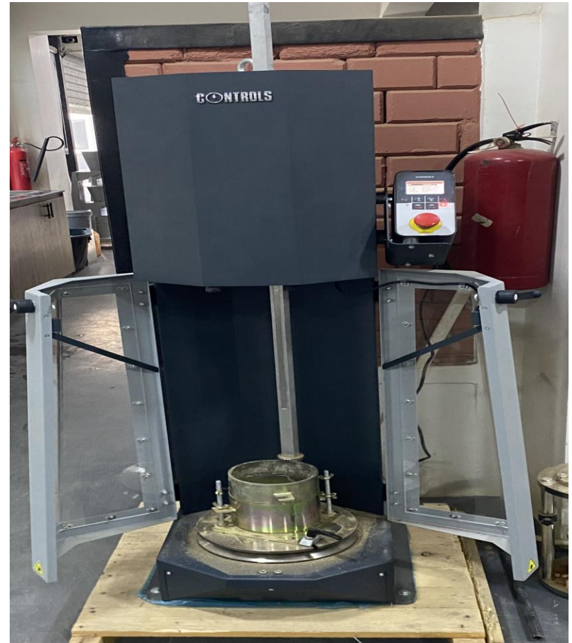
Plate III: Soil compaction for CBR test
